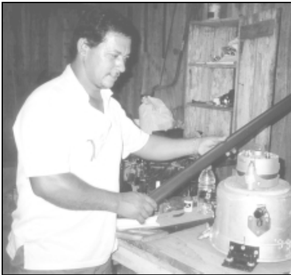
Franklin making final adjustments to the Pelton wheel assembly.
